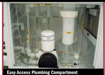
Easy Access Plumbing Compartment
